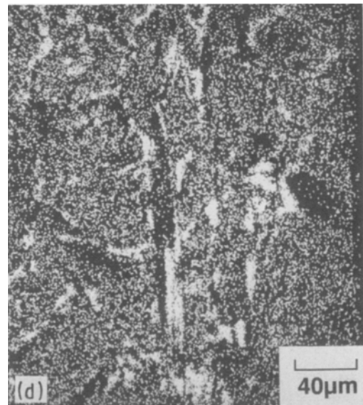
Figure 1 (a) Backscattered electron image and X-ray area scans of moderate-pressure-cast sectioned and polished metal-matrix composite, and distribution of (b) aluminium, (c) oxygen, (d) copper, (e) magnesium.
